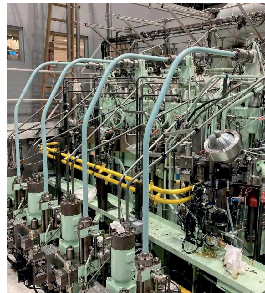
Successful ammonia combustion in a MAN B&W two-stroke engine marks an 'historic' step in the maritime sector. Image of the engine from MAN Energy Solutions.
